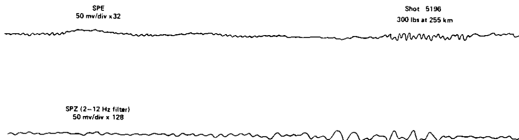
Figure 91-12. Comparison of the short-period east-west (SPE) and short-period vertical (SPZ) signals measured by the BIP from 300-lb. shot 5196, which was fired 255 km from GLOMAR CHALLENGER on the northwest refraction line of Figure 91-10.
