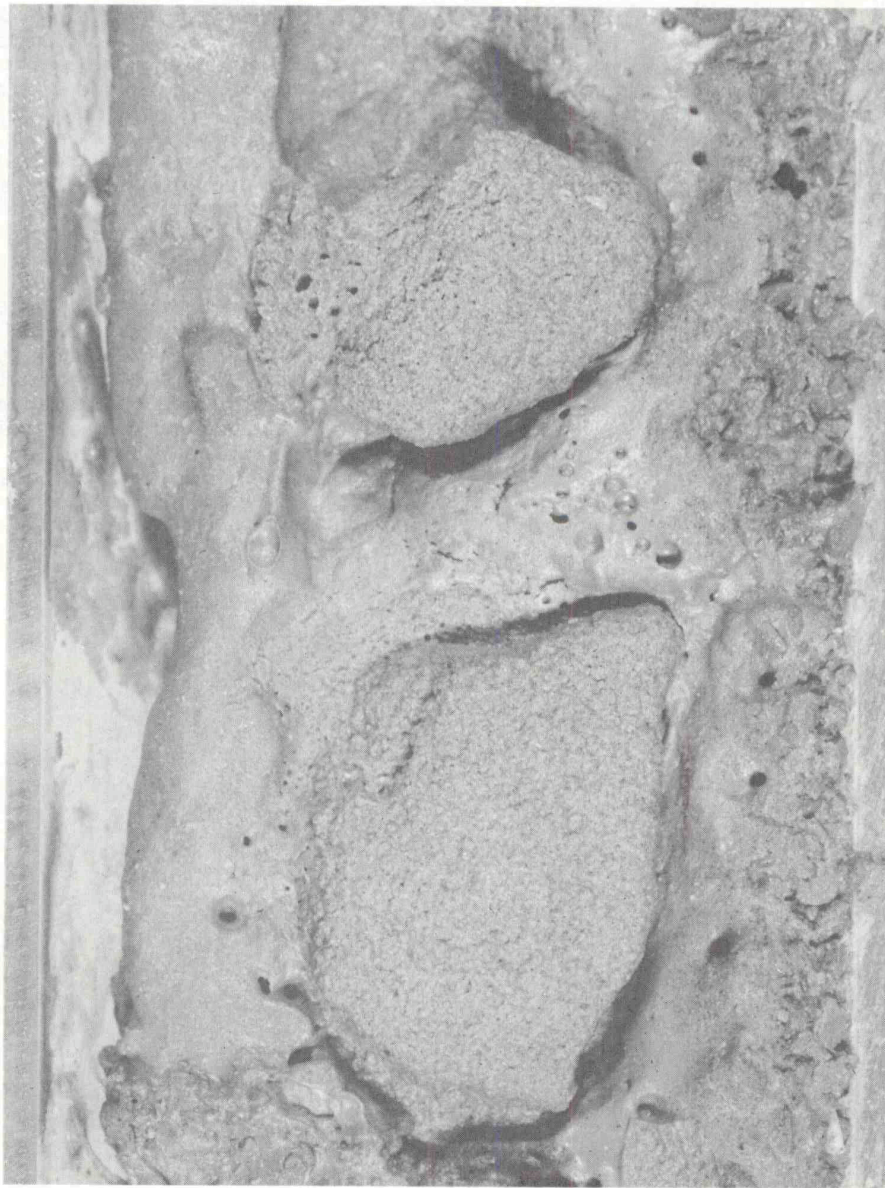
Figure 4: Hydrate-cemented vitric sand recovered in DSDP Hole 498A (Leg 67-Middle America Trench) - Sample 498A-15-2, 110-125 cms. As the hydrate melts, sand grains are incorporated into a clay-rich slurry. This shows the vents for gases released by the melting of the hydrates. [From Harrison, W.E. and Curial, I.A., 1982. Gas hydrates in sediments of Holes 497 and 498A. In Aubouin, J., von Huene, R., et al., Init. Rpts. DSDP, 67 : Washington (U.S. Govt. Printing Office), 351-382.]
