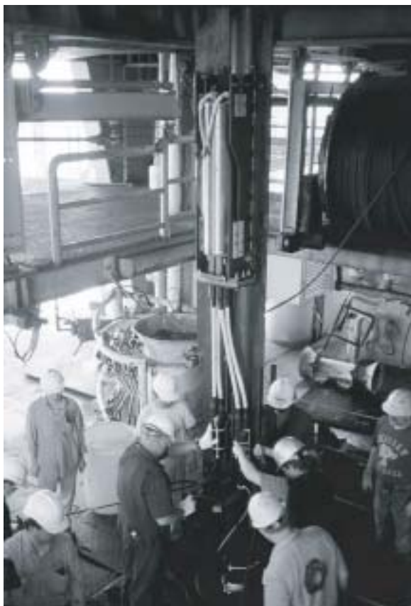
Figure 2 (left). Leg 195 Sewing Club attaching umbilical cables to stinger during ION seismometer deployment at Hole 1201D.
