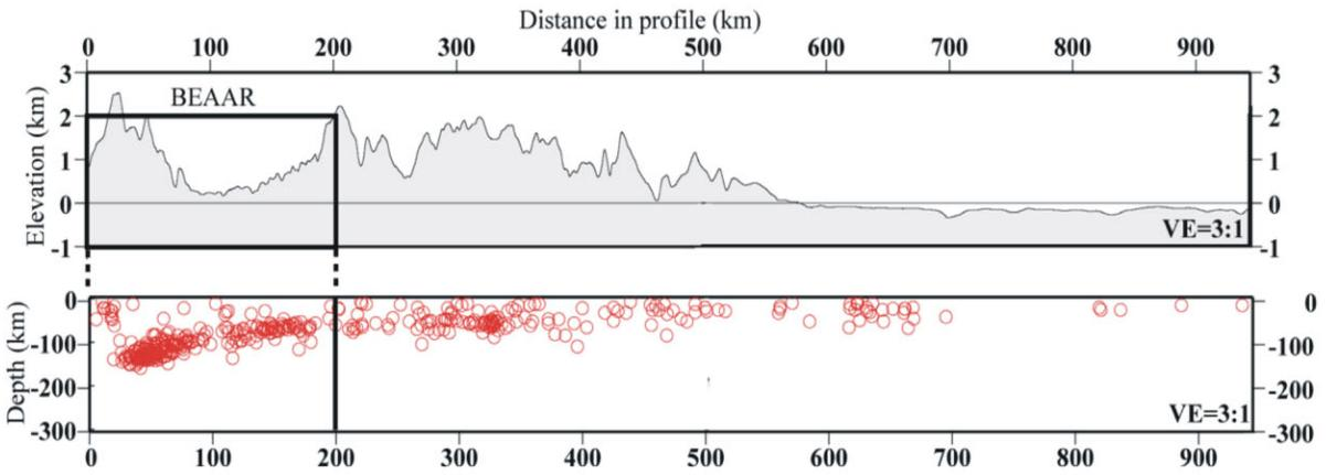
**Figure 9.** (Top) Topographic profile across southeast Alaska from the offshore Yakutat microplate to the northwestern limit of orogenic uplift. Approximate coverage for the BEAAR experiment (Ferris et al. 2003) is shown. (Bottom) Earthquakes along a 100-km swath centered on this profile from the NEIC catalog. Note the relatively flat subduction from ~200-600 km beneath southeast Alaska suggestive of a downgoing oceanic plateau. See Figure 10 for location of transect.
