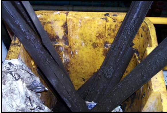
Figure 20. Discarded shattered liners.
