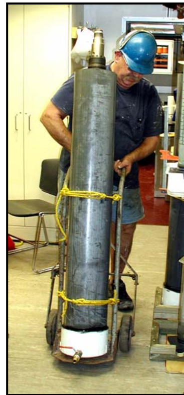
Figure 42. Pressure core barrel staying cool in ice container.
