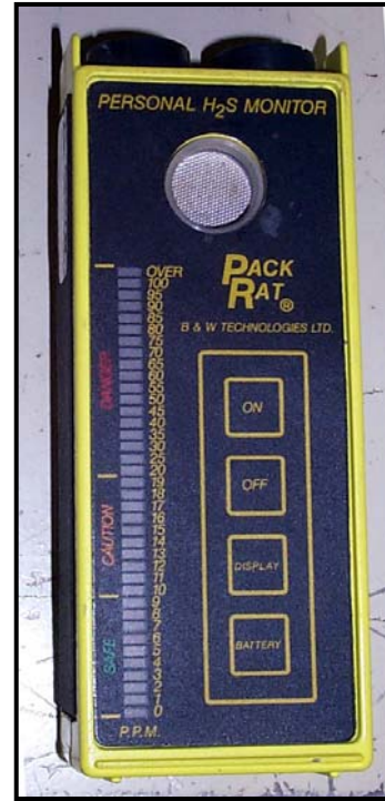
Figure 21. "Packrat" hydrogen sulfide (H 2 S) monitor.
