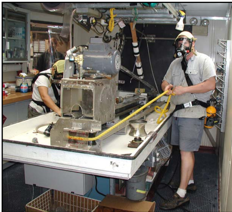
Figure 24. H 2 S core splitting.
