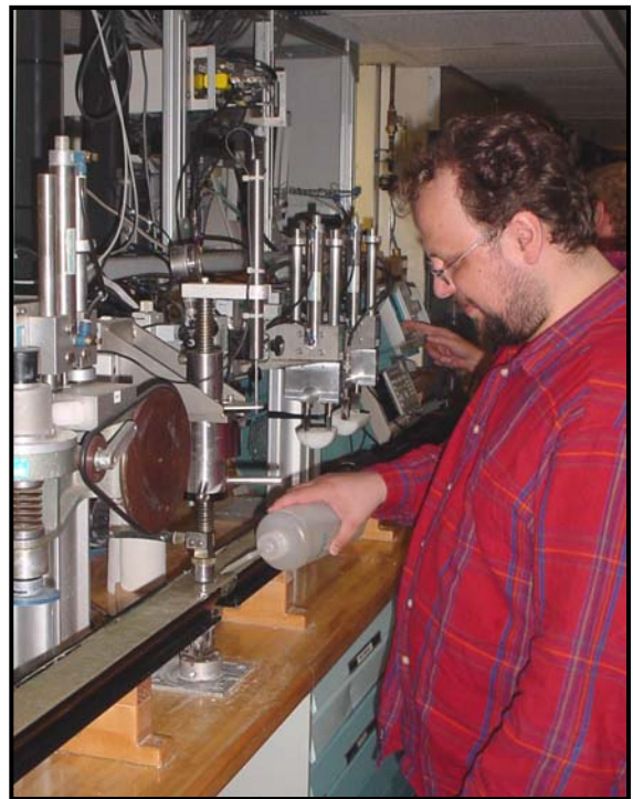
Figure 38. Measuring sonic velocity and shear strength.
