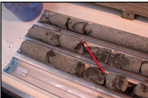
Figure 47. Hard rock ready for splitting line.
