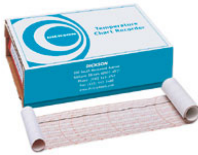
Figure 4. Disposable temperature chart recorder for refrigerated shipments.
