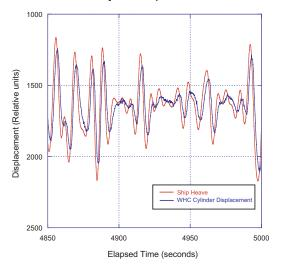
WHC performance data are routinely acquired during logging operations. Ship heave and WHC cylinder displacement are recorded and compared to evaluate WHC response to varying sea states.
