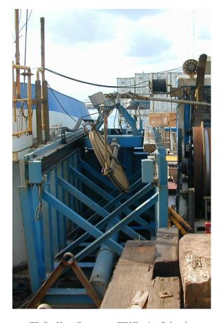
Wireline Heave Compensator (WHC) as installed on the *JOIDES Resolution*.
