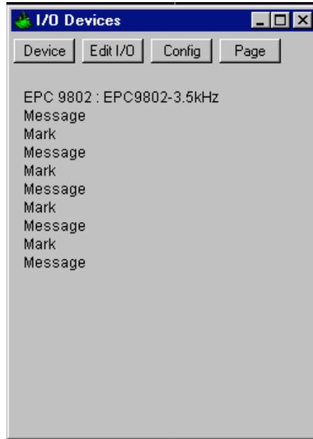
For the 3.5kHz, set the range to the whatever your current depth range is. Have messages set to print hourly, \_ hourly and 5 minutes. Set messages to print on the side opposite the bottom profile on the line scan recorder. The other parameters for the 3.5 should be set up as follows:
