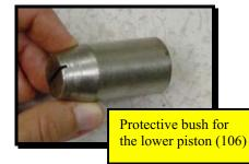
Screw the protective bush (picture) on the lower piston. Now you can carefully tap the piston 106 with the handle of the rubber mallet, if it does not want to come out by just pushing with your hand. DO NOT LET IT FALL OUT! If you have someone with you, ask this person to stand at the other end of the gun in order to hold on to the piston when it starts coming out.
