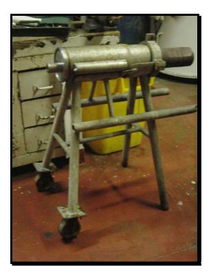
Push the cart over to the workbench. Again, have someone hold the damper while you detach it by removing the clamp. The damper is HEAVY too.
