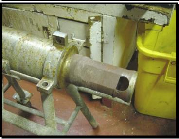
Re-assemble the damper. Put the clamps back on and secure them with the bolts.
