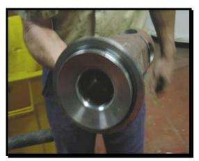
Now, pull out the solenoid valve block. The instructions for servicing the solenoid are on the PORT wall in the lab. Be gentle with it when pulling it out —do not go and scratch it with a wrench if it is stuck!
