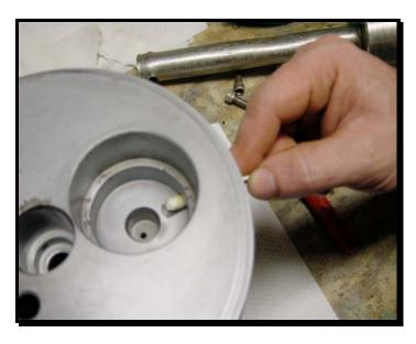
Clean the distributor with care, there are two O-rings 143 & 139 on the outside that you have to service, too. Remember to grease the holes on the end before you re-assemble the distributor.
