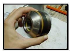
On the upper piston, there are an O-ring 142 and a split ring 132 on the outside, and an O-ring 140 on the inside. Clean all these and check their condition. Replace if needed, grease the piston and the O-rings. Remember to clean the piston wrenches before screwing the piston back in place, so you do not put any gunk from the dirty gun into the clean one.
