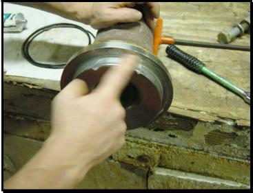
Clean the connecting surfaces and the O-ring 137 on the damper 122. Grease it, and grease the O-ring.
