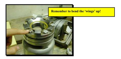
"Squeeze" out (look at the picture!) the two black O-rings 139 & 143 on the outside of the sleeve.
