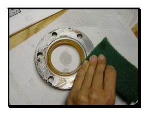
Clean the connecting surfaces between the clamp and the sleeve body well. Remove the yellow sealing ring 104.
