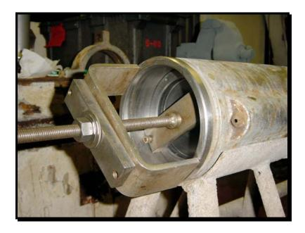
Now you have all the parts out of the gun body. It is time to start servicing them. We will take the sleeve 102 first. Place it on a piece of paper towel. Clean it well. Use oil or grease if needed, and a green scrub pad. Make sure not to scratch it.
