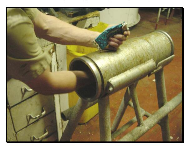
Next, take off the black split ring 107 and the O-ring 137 on the lower piston 106. Clean the piston and then grease it well. Do not forget to grease the shaft. Check for damage on the rings and replace if needed. Clean, grease properly and put back in place.
