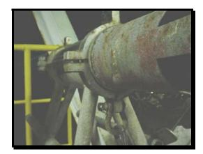
Remember to put the O-ring 143 between the distributor and the tail. Reassemble the tail and put the clamps back on.
