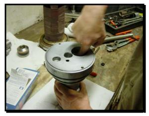
When re-assembling, pay attention to the holes lining up horizontally (the solenoid hole to the right!), or you will be in trouble later.
