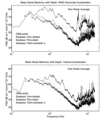
Comparisons of SEABASS and OBS spectra for horizontal (above) and vertical (below) components show that borehole sensors are generally quieter than seafloor sensors from 0.3-20Hz.
