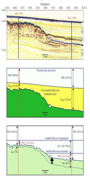
W1=present day water depth; S=thickness of postmiddle Miocene sediment load; PW=paleowater depth estimated from biotic assemblage; De=sediment expansion (reduced water depth); DSL=magnitude of eustatic fall.
