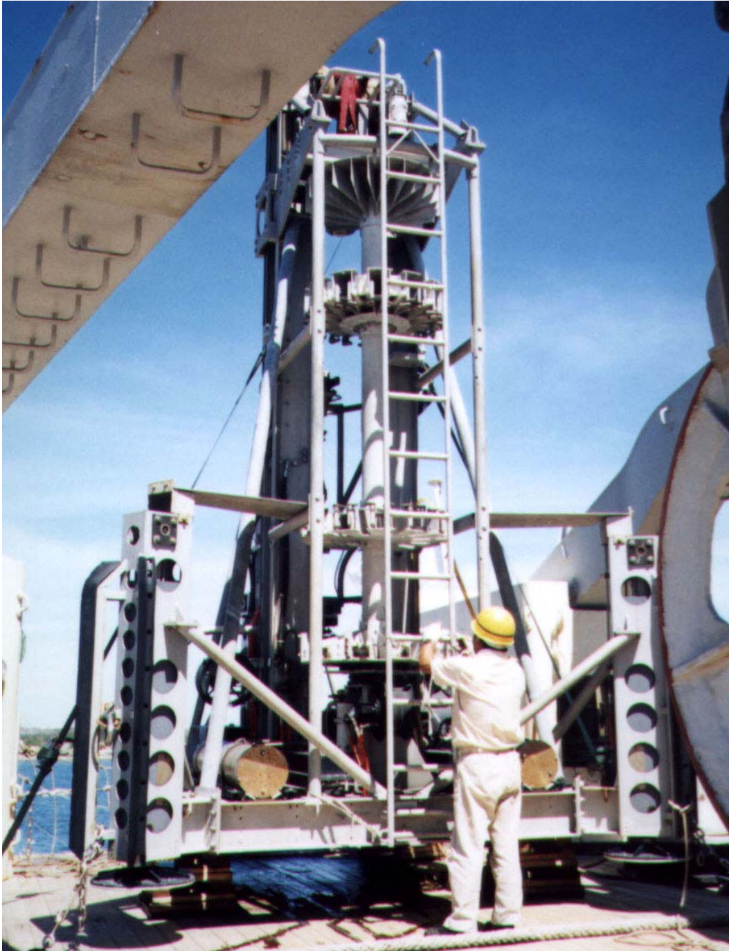
Figure 2. Benthic Multicoring System (BMS) drill, built by Williamson and Associates, Inc. for the Metals Mining Agency of Japan. The BMS is 5.9 m in height and weighs 5 tons in air. It is designed for up to 6000 m depths and can take 20 m of 48-mm diameter core in 2.2 m sections.
