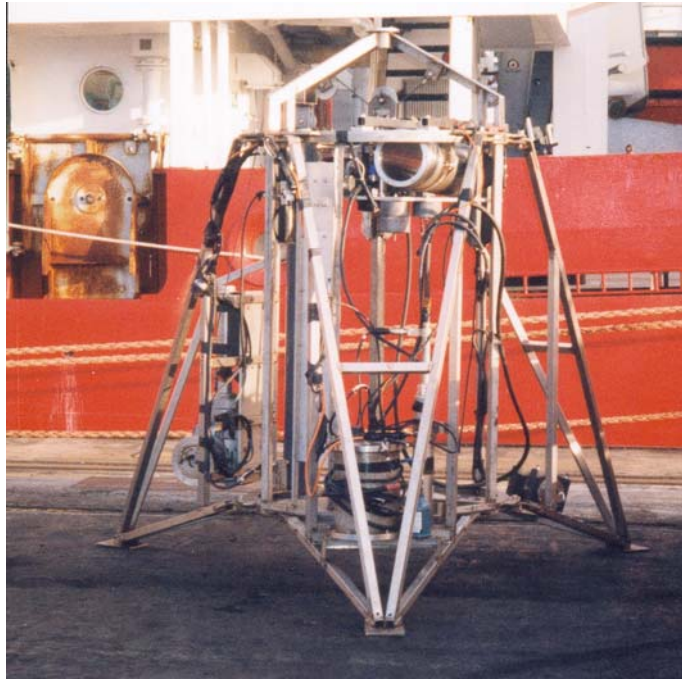
Figure 6. British Geologic Survey 1-m BRIDGE drill. The device is approximately 1.5 m in height and weighs 900 kg in air. It operates from a standard 0.68-in coaxial cable, can recover a 35-mm diameter core ~1m in length, and has been used to depths of 4500 m (see Allerton and Tivey, 2001; MacLeod et al., 2002).
