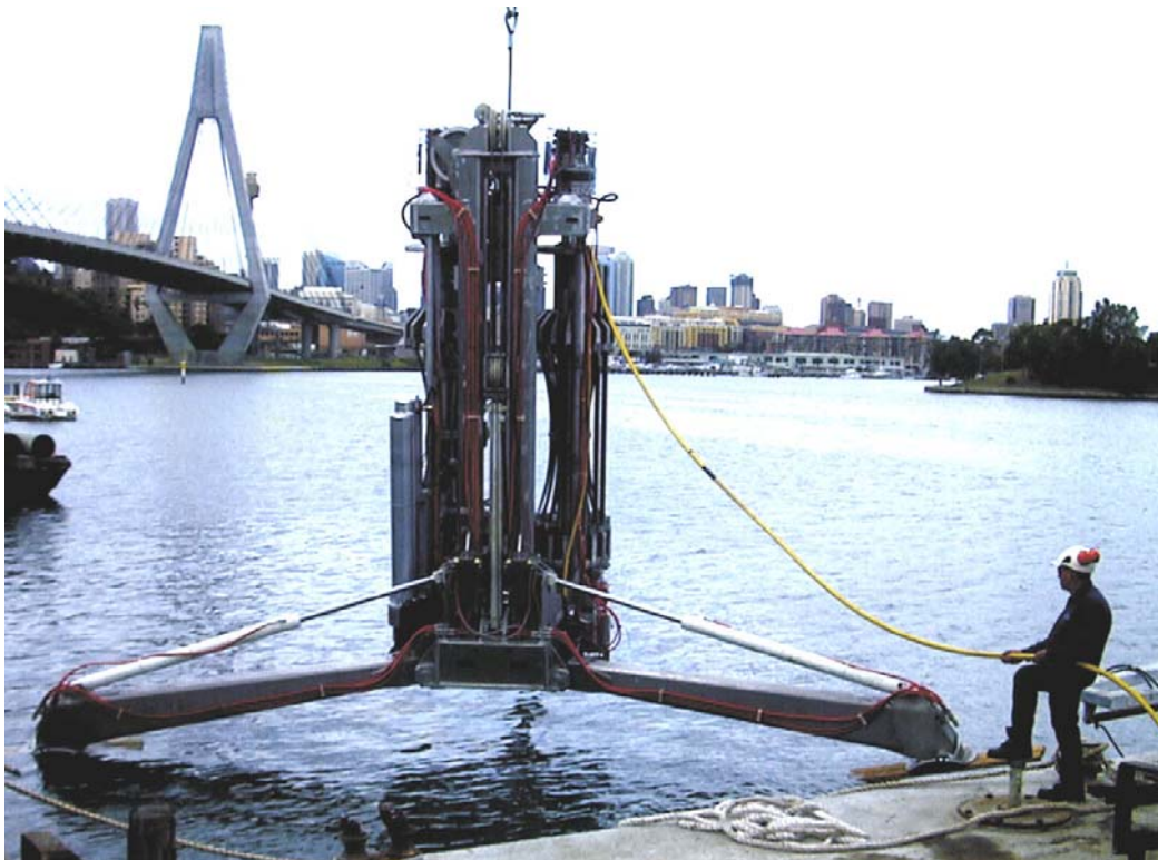
Figure 3. Portable Remotely Operated Drill (PROD), constructed by Benthic GeoTech Pty, Ltd. (Australia) in cooperation with Williamson and Associates, Inc. This drill is 5.8 m in height and weighs approximately 10 tons in air. It can drill up to 100-m penetration depth by assembling a drill string from pipe segments carried in a rotary magazine. (see http://www.bgt.com.au/prod.htm )
